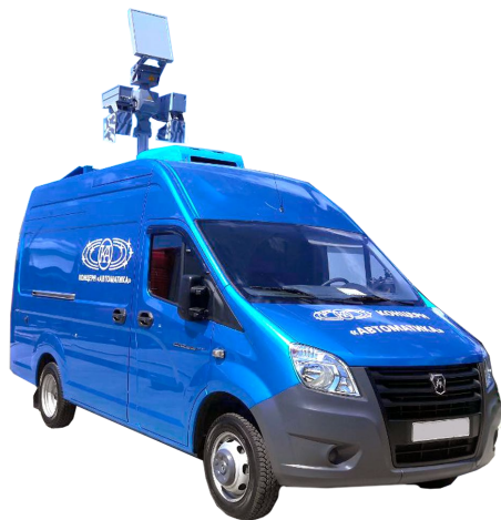
UAV detection and counteraction mobile complex "Sapsan-Bekas"
