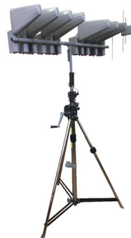
Radio-electronic suppression "Luch" module (targeted action in frequency and direction)
